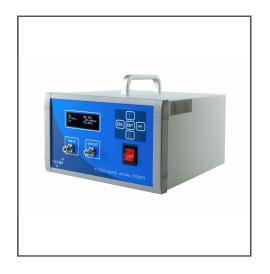
The Rapidox 1100H is a cost-effective hydrogen ( $H_2$ ) gas analyser fitted with a durable thermal conductivity (TCD) sensor. Specifically designed to analyse  $H_2$  in percent measurements, the Rapidox 1100H is ideal for applications such as glove boxes or research and development.
