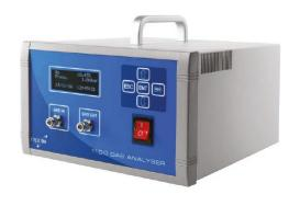
The Rapidox 1100Q is a cost-effective helium (He) gas analyser fitted with a durable thermal conductivity (TCD) sensor. The sensor is carefully heated to 50°C to prevent any ambient temperature changes causing drifting. Specifically designed to analyse He in percent measurements, the Rapidox 1100Q is ideal for applications such as gas generation, cooling, inert gas blanketing, leak testing, welding & diving.
