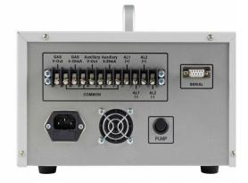
This principle is very robust. It shows virtually no interference to other gases, has a very low drift, and the sensor is fully solid-state. It does not deplete over time, unlike galvanic oxygen sensors with their limited shelf life. Optics and electronics are hermetically sealed from the measured gas. For typical indoor environmental conditions, a five year operating life is expected.
