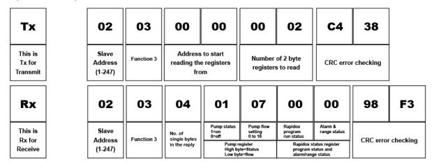
Figure 14: Example of a typical function 3 transmission and receive
