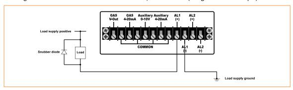
Figure 7: Analogue Output Connections: AL1 & AL2
