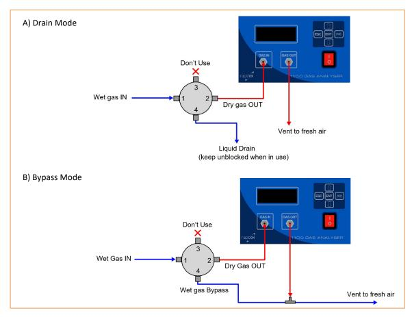
Figure 6: Examples of how to set up and use a water membrane filter on gas lines that have a lot of liquid water present
