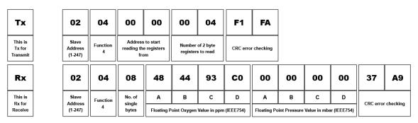
Figure 15: Example of a typical function 4 transmission and receive
