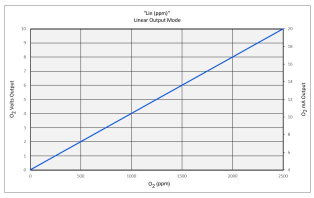
Figure 9: Graph showing the linear output mode option for oxygen
