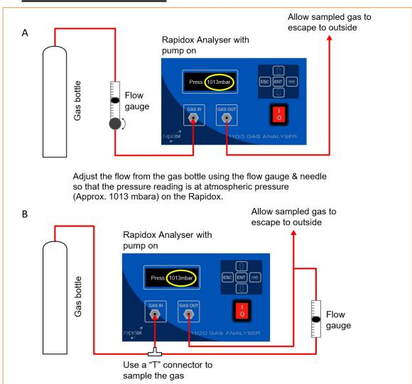
Figure 8: Examples of a typical calibration setup
