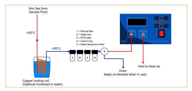
Figure 5: Making the gas connections to filters & dealing with cooling down hot gas
